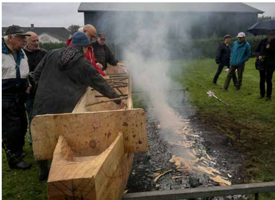
Figure 11. Photo of The Hjortspring laug (The Hjortspring boat building team) expanding the log boat Bjørkebåten with heat and fire. A similar technique must have been used when expanding the hull, the bottom plank for planked built boats such as the Hjortspring type or Dover type. Photo by members of The Hjortspring laug.
