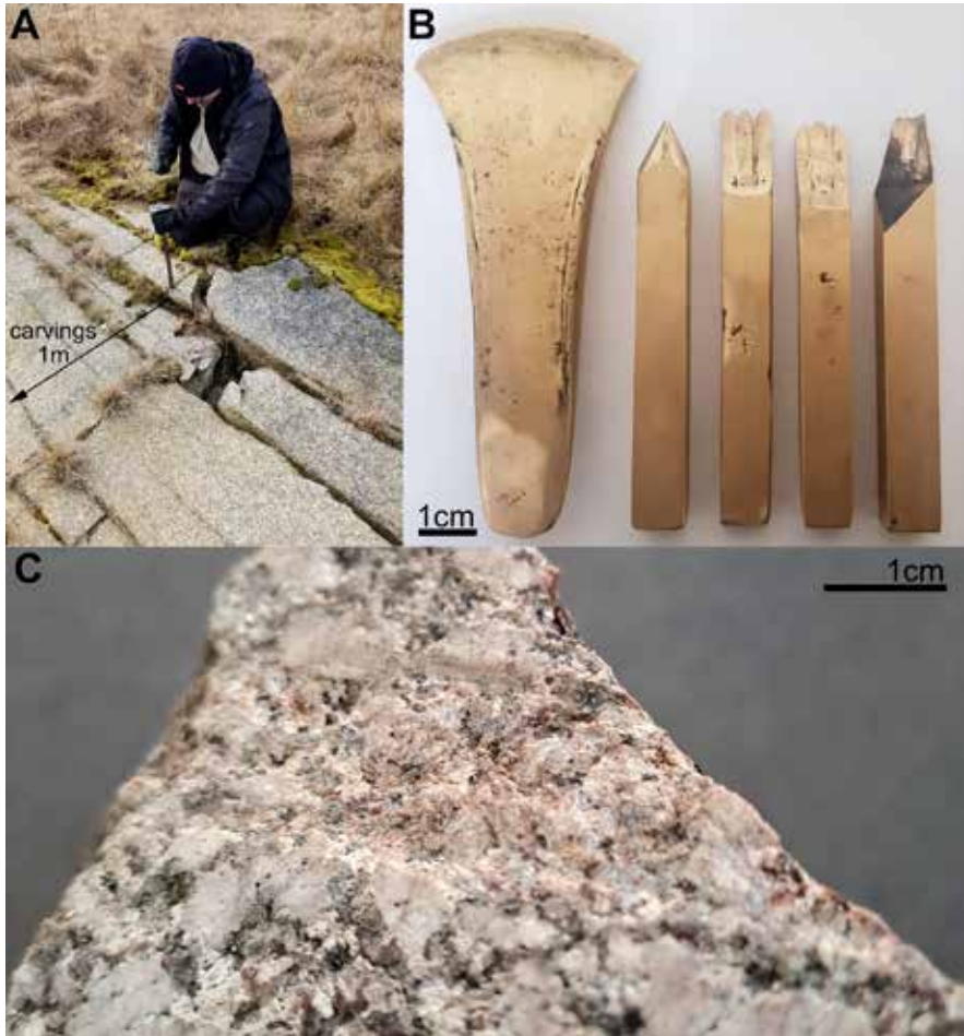
Figure 4. Photographs from carving experiments using bronze tools on a polished rock sample of the Bohus granite. (A) Rock sample TH-02 taken at the side of panel Tanum 190 approximately 1m next to carvings (B) Replicated Bronze age axe head and various shapes of chisels made of bronze (C) carving done with bronze tools and hammerstone. Photos: Carina Liebl
